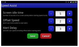
When the set speed has been exceeded for the time and the offset, the screen will flash red and an audible alert will sound.
